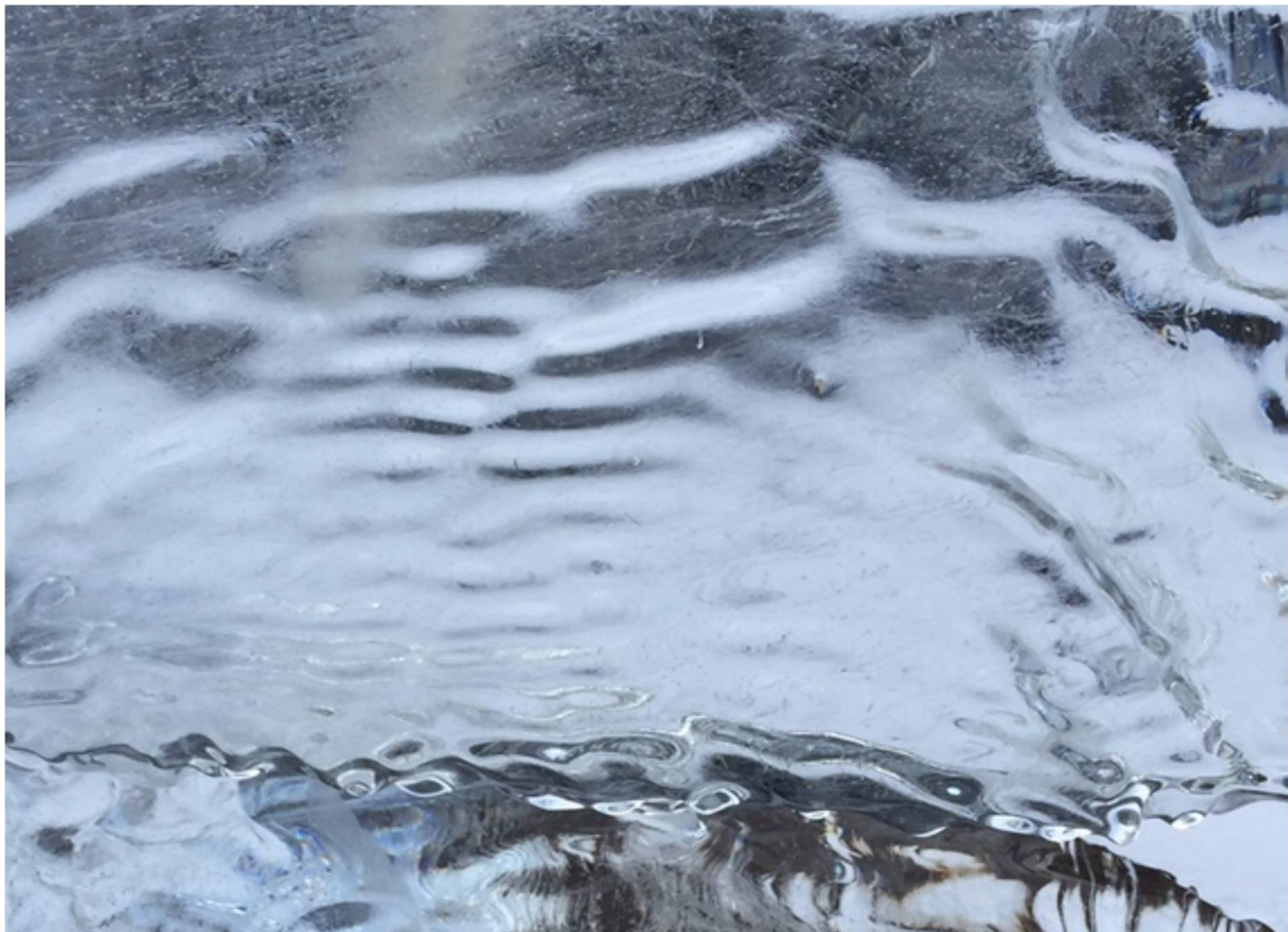
Ice after propane flame at 6 bar 2 million BTU/hour
